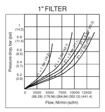
Flow graphs are for 40µm filterations only
